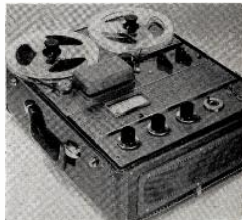
NEW AMPEX 600 professional recorder weighs less than 28 pounds, can be used with line or microphone outputs.
